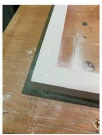
The image on the left shows the missing bits of paint resulting from the cutting process necessitating gap filler, sanding and repainting.
